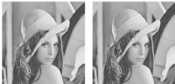
(a) tile=64 pixel×64 pixel, M=64 , Br=0.25 bpp, PSNR=31.65 dB (b) tile=128 pixel×128 pixel, M=16 , Br=0.25 bpp, PSNR=33.74 dB
