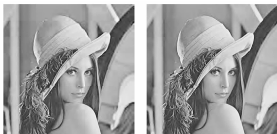
(c) tile=64 pixel×64 pixel, M=64 , Br=0.25 bpp, PSNR=32.15 dB (d) tile=128 pixel×128 pixel, M=16 , Br=0.25 bpp, PSNR=34.38 dB
